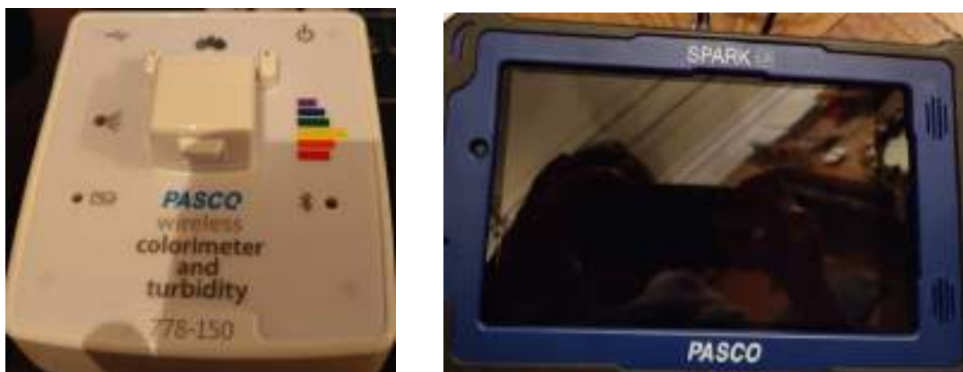
Fig.5 PASCO Wireless colorimeter and turbidity meter
