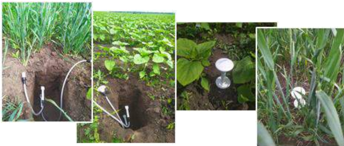
Figure 2.4: Soil temperature & moisture loggers TOMST installed in sunflower and winter wheat fields within the PONTOS-UA pilot.
