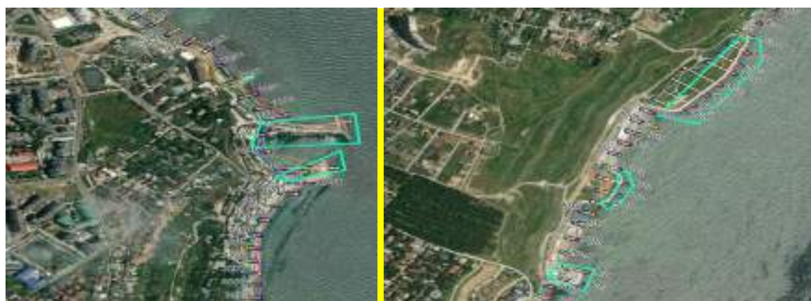
Fig. 3.15. Hydro-engineering structures of the marina in Chornomorsk. Light-blue polygon outlines show the sites for which wrong result was obtained in the previous calculations of coastline displacement (left) and man-made cape landforms of landslide prevention works in village Fontanka. Light-blue polygon outlines show the sites for which wrong result was obtained in the previous calculations of coastline displacement (right).
