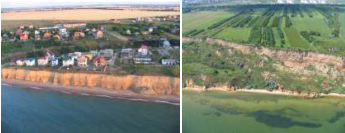
Fig. 2.6. Abrasion-avalanche type of coast (left-side picture) and Abrasion-landslide type of coast (right-side picture)..
