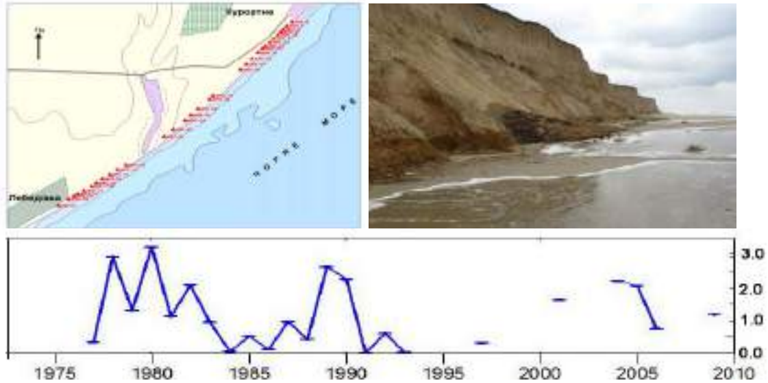
Fig. 2.9. Abrasion monitoring Station “Lebedivka” at the Black Sea coast between the Burnas Lake (Lebedivka village) and the Budak Estuary (Kurortne village). On top – scheme of the monitoring station (the triangles show the benchmarks and their numbers) and a photo of the coastal slope; at the bottom – the average for the site cliff edge retreat rate (m/year).
