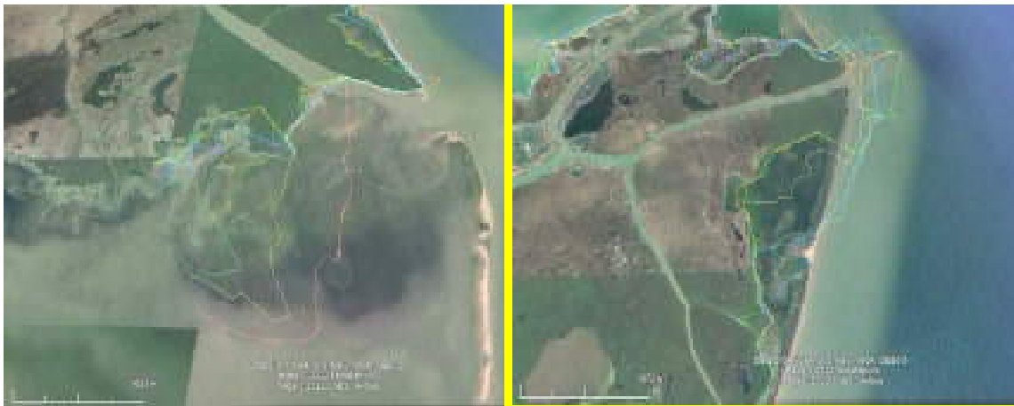
Fig. 3.11 Wrong positions of coastlines in the UA1-1 subarea from 0.0 km to 3.18 km (left) and from 31.56 km to 31.82 km (right).
