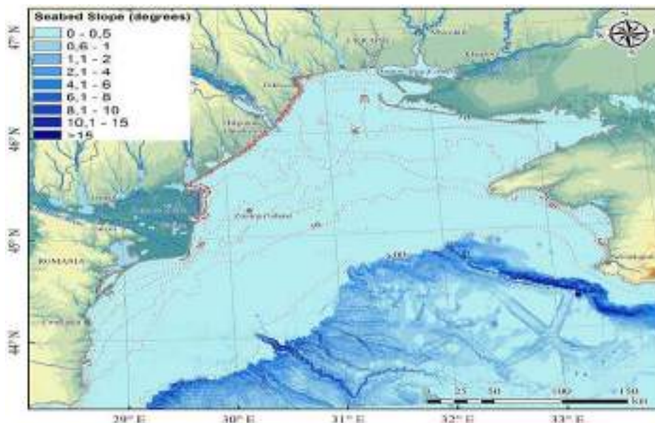
Figure 4.2. Bottom slopes in the north-western part of the Black Sea. Source: the EMODnet Digital Terrain Model (DTM), version of 2020, https://portal.emodnet-bathymetry.eu/
