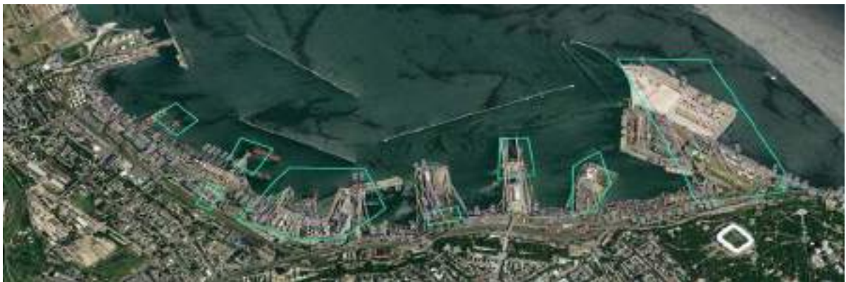
Fig. 3.14. Odessa Port's berthing facilities. Light-blue polygon outlines show the sites for which wrong result was obtained in the previous calculations of coastline displacement.
