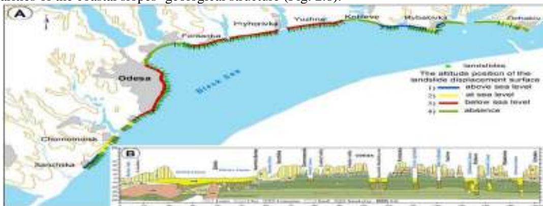
Fig. 2.8. The area of the northwestern Black Sea coast with abrasion-landslide shore type, where mainly landslide processes prevail (A) and the corresponding alongshore geological & lithological section (B) [Cherkez et al, 2021].
