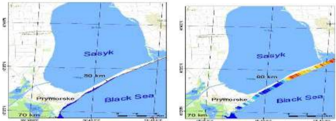
Figure 5.10. Maps of coastal area change near Sasyk estuary (UA1-2 subarea) . Left – Dynamics of shoreline for 1980-2020: ■ Erosion, ■ Accretion. Right – Distribution of WLR (Weighted Linear Regression Rate) for 1980-2020, m/year: — High Erosion ( < -2 m/year), — Medium Erosion ( -2 - -0,5 m/year), — Stable Coastline ( -0,5 - 0,5 m/year), — Medium Accretion ( 0,5 - 2 m/year), — High Accretion ( >2 m/year).
