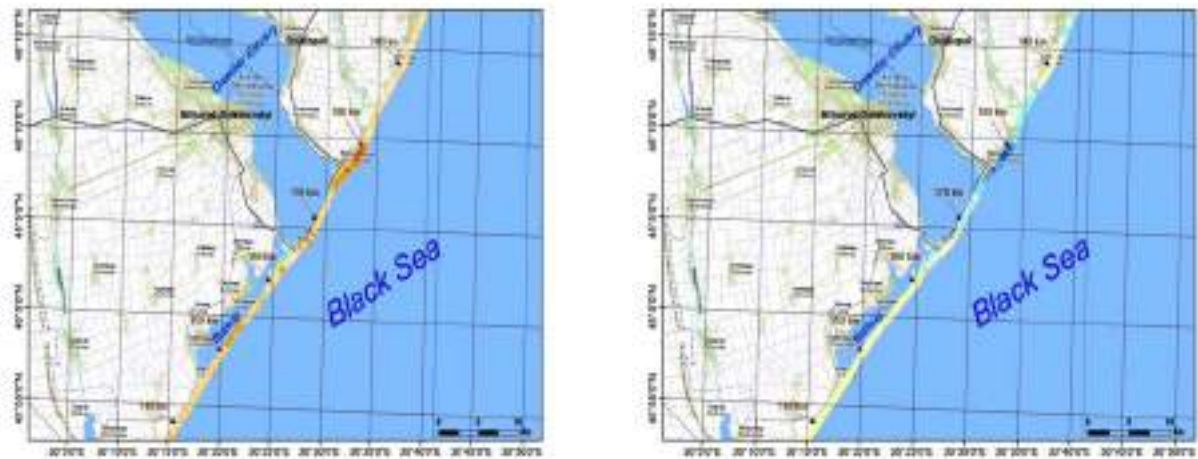
Figure 5.26. Statistical parameters SCE (left) and NSM (right) by transect along the shoreline for subarea UA1-4 (Budakskiy estuary - Sukhiy estuary) for the period 1980-2020. Red arrow km distance; For SCE: White 0-20 m, Light Yellow 20-50 m, Yellow 50-100 m, Orange 100-250 m, Dark Orange 250-500 m, Red 500-1000 m, Dark Red >1000 m. For NSM: Red < -250 m, Orange -250- -100 m, Yellow -100 m- -20 m, White -20- 20 m, Light Blue 20- 100 m, Dark Blue 100-250 m, Dark Blue >250 m.
